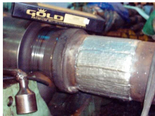
Worn shaft reclaimed by welding with NSB-312
