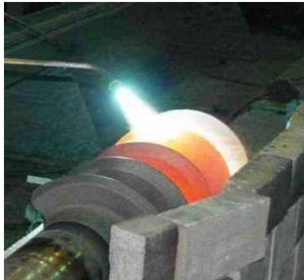
Coating of Screw with WC Powder 2070 Using spray and fuse torch 2010
